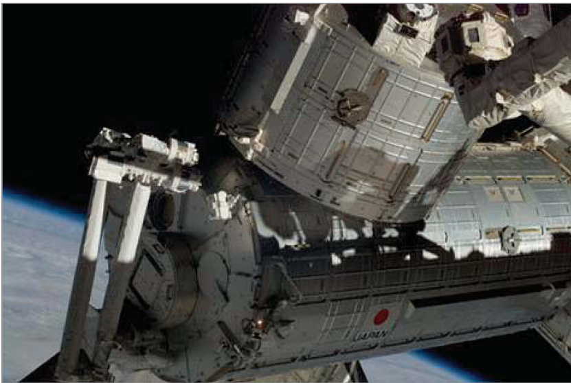
Fig 57: The above Pressurized Module, installed on the ISS during the STS-124 Mission (bottom) https://iss.jaxa.jp/en/kibo/about/kibo/jpm/
